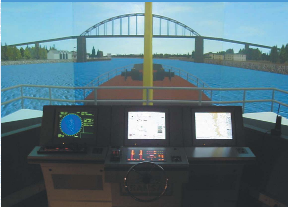
A modern radar navigation simulator at the Faculty of Maritime Studies in Rijeka
