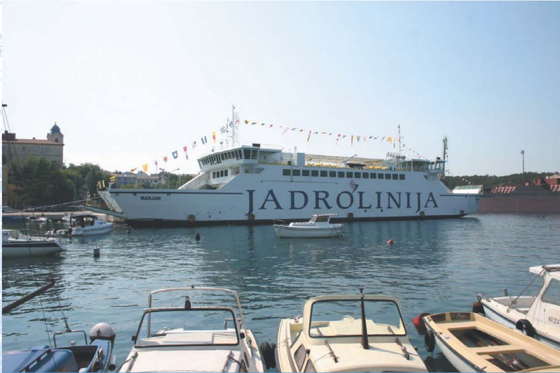
M/V Marjan – Jadrolinija – Rijeka – the largest ferry built in a Croatian shipyard for a domestic shipping company, capacity 130 vehicles and 1200 passengers; built within the state subsidized program for rebuilding and developing the Jadrolinija passenger fleet in the 2004-2008 period
